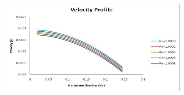
The above graph shows velocity profile of a non-Newtonian fluid flowing between two infinite porous plates which are placed in an inclined magnetic field. It appears from the graph that velocity decreases with increasing magnetic field for all values of Reynolds number. For lower value of Reynolds number the velocity adopts lower values and vice-versa and thus the pattern remains the same.
