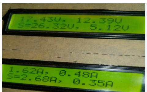
Plate4. LCD display for voltage and current reading
