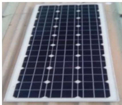
Plate2. 24V/100W Solar Panel
