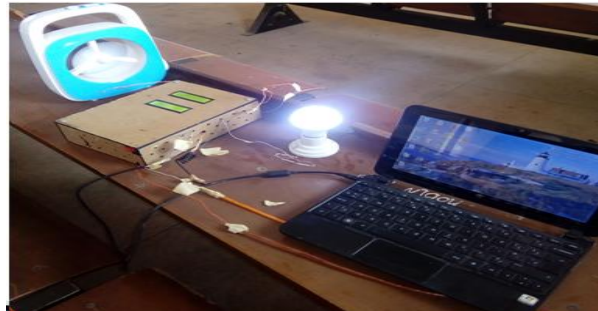
Plate5. The unit powered all three devices ( a 19V Laptop, 12V bulb and 5V fan)
