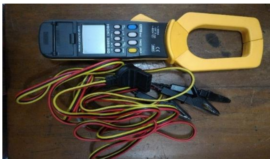
Fig4. Power Quality Analyzer
