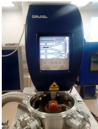
**Figure9.** Installation of the test samples in a vacuum chamber at Polytec MSA-500
