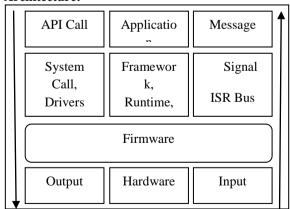
Hardware refers to physical chips soldered to iphone circuitry. Firmware refers to chip specific code that is either contained in with memory in/around the peripheral itself or within the drive for said peripheral. Processor refers to ARM Instruction set
