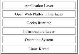
Application layer consists of user interface implementation based on building blocks and JS libraries. Web Platform Layer provides runtime and middleware that provide capabilities needed by the application layer. Infrastructure layer provides the lower level Operating system services, libraries and other infrastructure services based in linux and other open source software. It also provides security ad privacy. "Gecko Runtime" is the application runtime of firefox operating system.
