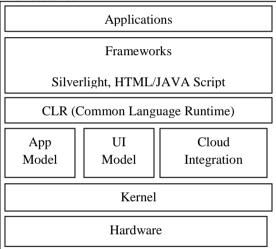
The Hardware is composed of ARM 7 CPU, Direct X 9 Capable GPU, 256 MB RAM, Capacitative multi touch display with required Physical buttons. Kernel Handles low level device driver access as well as basic security, networking and storage. The three libraries App Model, UI Model and Cloud Integration Model sit above the kernel for application management and notifications. Application facing APIs include silver light, HTMI/Java Script and CLR that supports C#.Net and VB.Net applications.
