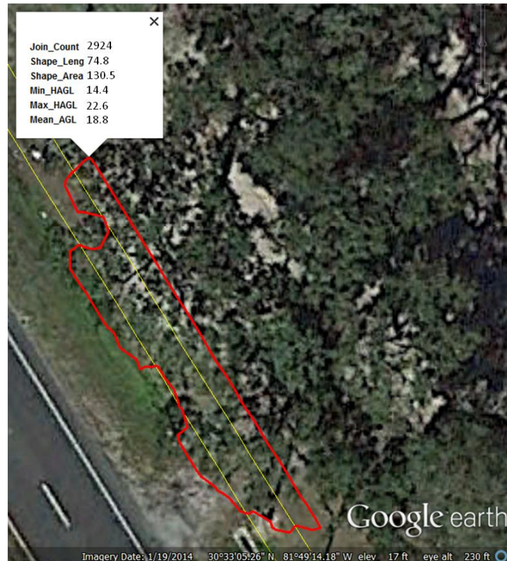
Figure25. A vegetation encroachment polygon displayed in Google Earth with HTML popup showing attributes
