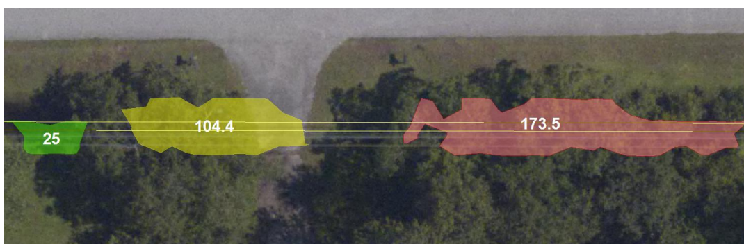
Figure24. Vegetation encroachment polygons symbolized and labeled according to their areas in meters
