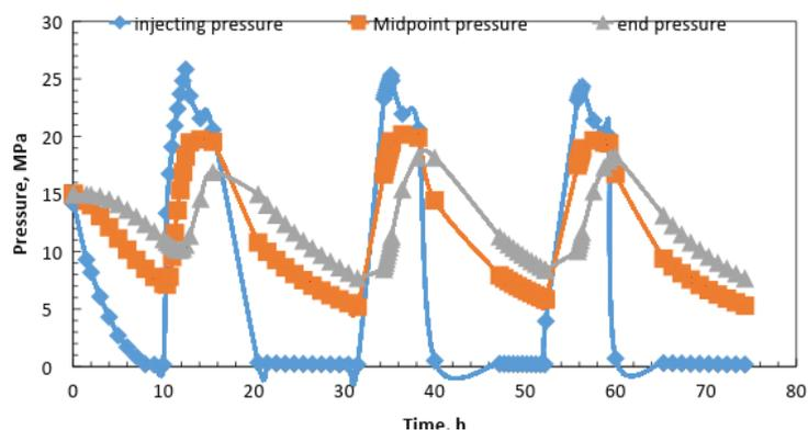
Figure10. Pressure of midpoint and terminal point in injecting gas
