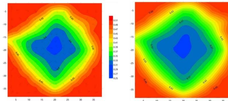
Figure12. Oil saturation field at the end of first round and the second round
