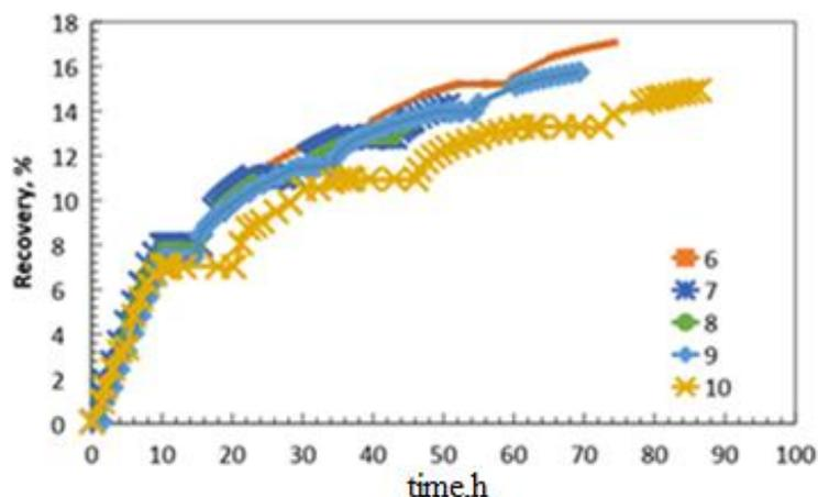
**Figure7.** Relationship between recovery and gas injection time
