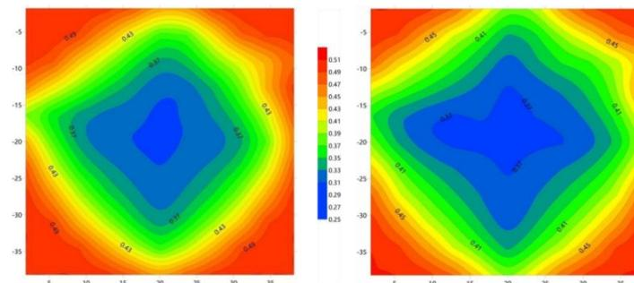
Figure13. Oil saturation field at the end of second round and the third round
