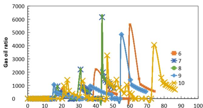
Figure8. Relationship between gas oil ratio and gas injection time
