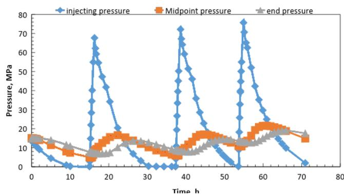
Figure9. Pressure of midpoint and terminal point in injecting water
