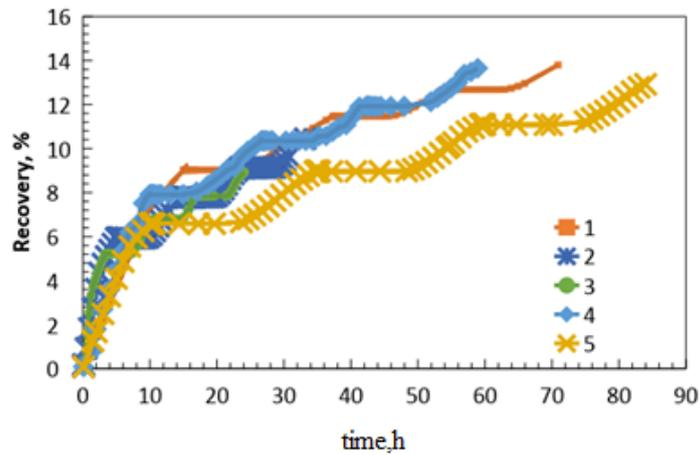
**Figure3.** Relationship between recovery and water injection time
