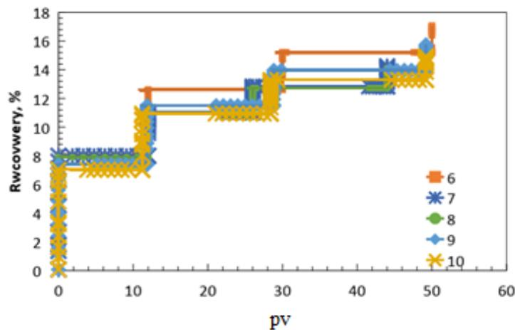
**Figure6.** Relationship between recovery and gas injection pore volume
