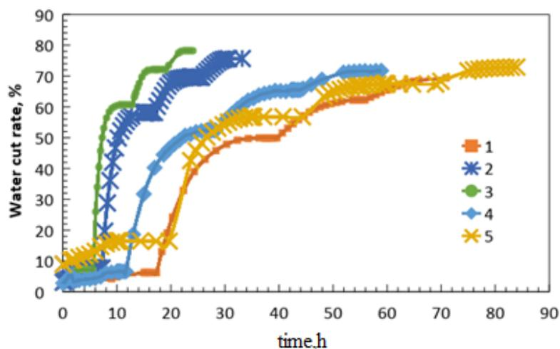
**Figure5.** Relationship between water cut rate and water injection time
