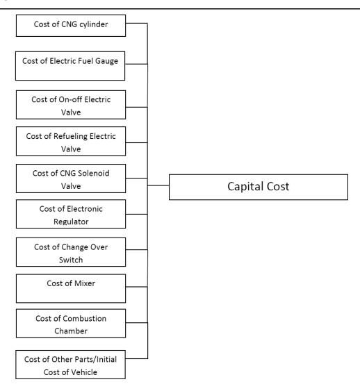
Fig2.2. Economic flow chart for manufacturing CNG-powered vehicles
