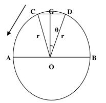
Let, r be the radius i.e. OA = OB = r and  $\angle GOD = \theta$ Let, the cutting width,  $CD = 2\Delta x$  i.e.  $GD = GC = \Delta x$  $\therefore$  Total number of cuts required  $= 2\pi r/\Delta x$
