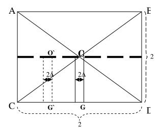
Cutting movement will be vertical i.e. parallel to  $\xrightarrow{AC}$  or  $\xrightarrow{BD}$  direction. Here, one conveyor belt will be placed in the direction  $\xrightarrow{OO}$ .
