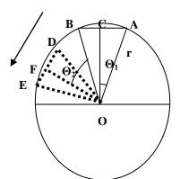
Let, r be the radius i.e. OA = OB = r and  $\angle BOA = \theta$ Let,  $\triangle DOE$  be the p<sup>th</sup> slice.  $\therefore \angle BOE = p\theta$ Let, the cutting width AB or DE be  $2\Delta x$ .
