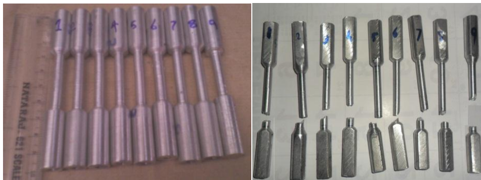
Fig3. Tensile test specimen before testing and after testing
