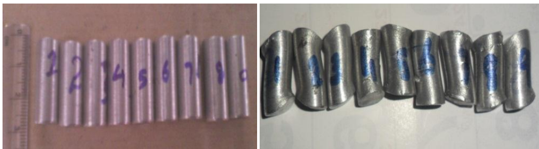
Fig4. Compressive test specimen before testing and after testing
