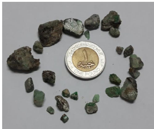
Fig 8. Some of beryl grains associating with phlogopite schist from the mine dumps at W. Zabara area, SED, Egypt.
