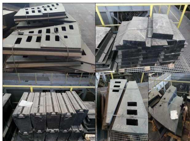
Figure2. View of the rubber liners, lifters and discharge grate
