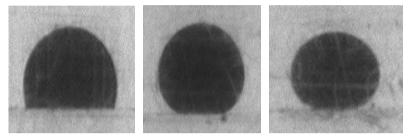
a.Brineb. carbon nano particlesc. SiO2Figure4. Contact angle test results with different type of fluids.
