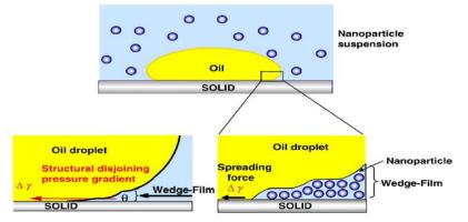
Figure 2. Nanoparticles establishing a wedge film, resulting in a structural Disjoining pressure.[16]
