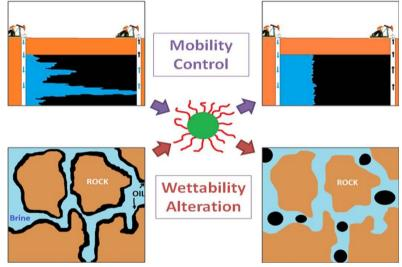
Figure 1. Schematic for the application of PNPs in EOR through mobility control and wettability alteration[2]
