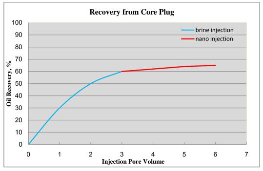
Figure5. Oil recovery results for water flooding and nano fluid injection
