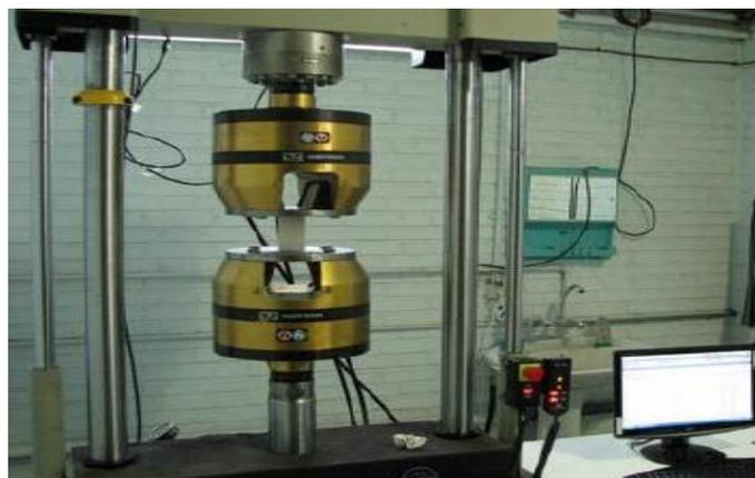
**Figure3.** INSTRON 8802 servo-controlled testing equipment
