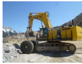
Figure 1. Base frame and stub axels of a sleipner shoe. Figure 2. Hydraulic excavator pulling into a pair of sleipner shoes.
