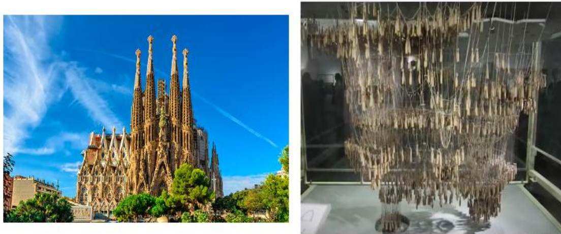
Fig9. Sagrada Familia(left) and Gaudi's designing experiment using strings and sandbags (right). (in public domain)
