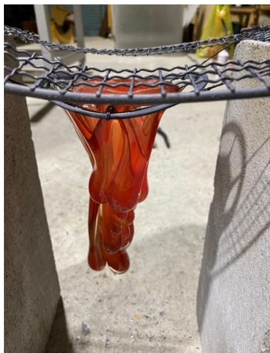
Fig7. An example of melted glass sagging down from a mesh.
