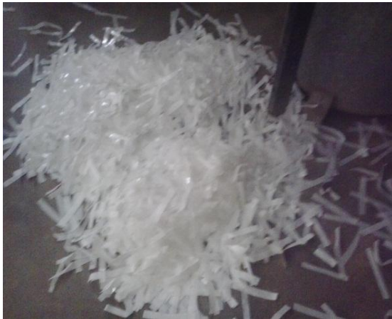
Plate I. Cut Polythene fibre (10mmX50mm)
