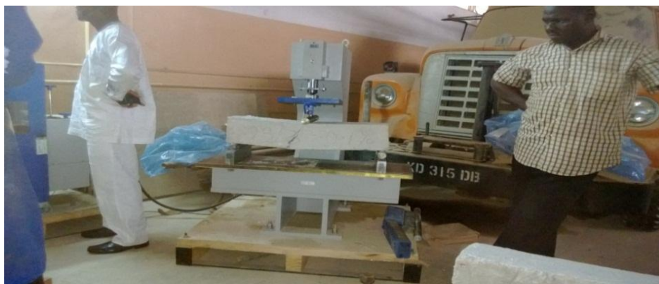
Plate III. Bending test on Beams [19]
