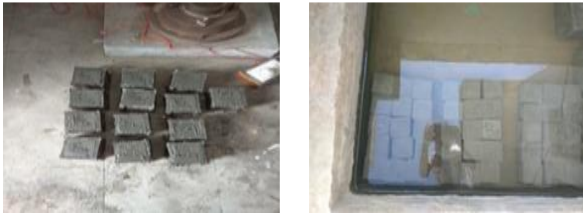
Figure5. Casting and curing of cement mortar cube
