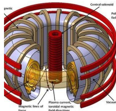
**Figure5.** Closed plasma trap (tokamak).
