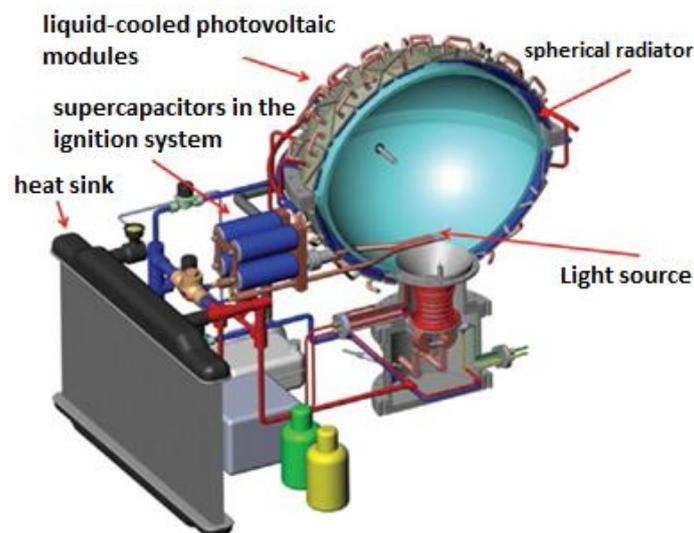
Figure7. SunCell device diagram ("solar cell")
