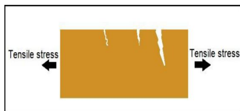
Figure6. Stress cracking corrosion
