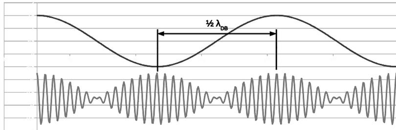
**Figure3.** The de Broglie wave (top) and the real part of (17) plotted against  $x'$  for  $t' = 0$ ,  $y' = z' = 0$  and  $\beta = 0.0345$ , an example where the spherical wave model leads to constructive interference in screen regions where the de Broglie wave alone interferes destructively.
