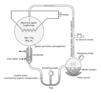
Fig1. Miller-Urey experiment setup
