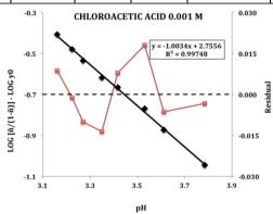
Figure5. Bilogarithmic method for the potentiometric evaluation of pKa of chloroacetic acid
