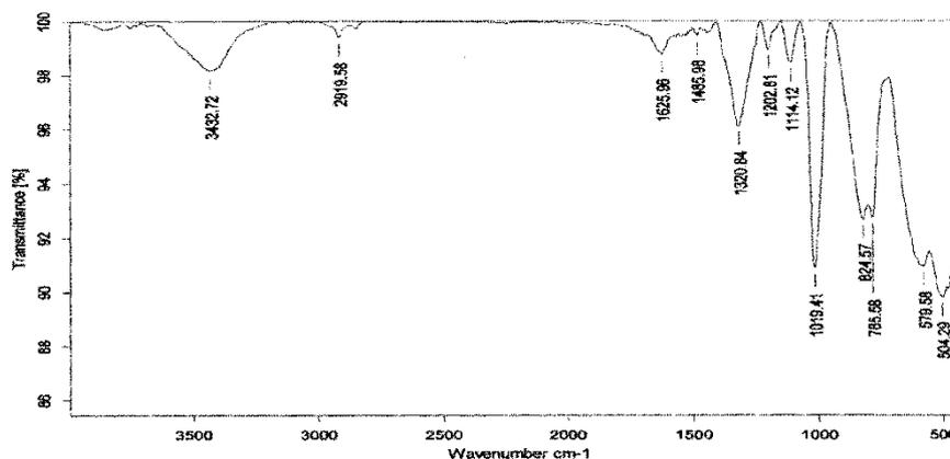
Figure1(b). FTIR spectra of PTh /1 %w/v V<sub>2</sub>O<sub>5</sub> composite thin films
