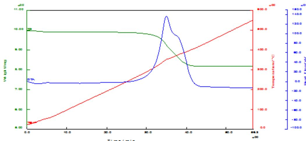
Figure4(b). TGA-DTA of polythiophene 1%w/v V<sub>2</sub>O<sub>5</sub> doped
