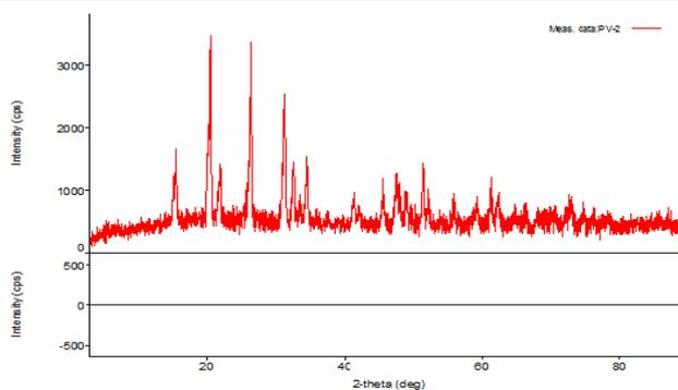
**Figure2(b).** XRD patterns of Polythiophene 1% w/v  $V_2O_5$  doped composite.
