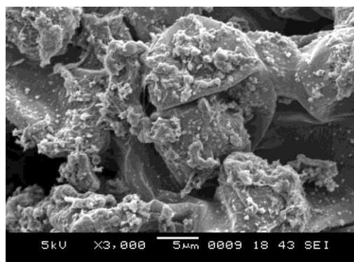
**Fig3(a).** SEM image of 0.5%w/v  $V_2O_5$  doped polythiophene thin film.
