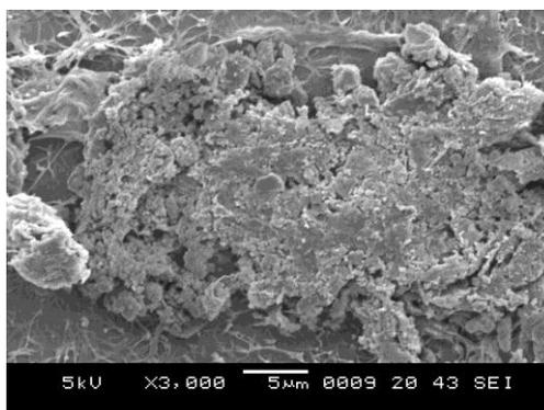
**Figure3.** SEM image of undoped polythiophene thin film
