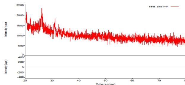
Figure2(a). XRD patterns of polythiophene 0.5% w/v V<sub>2</sub>O<sub>5</sub> doped composite
