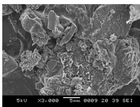
**Fig3(b).** SEM image of 1%w/v  $V_2O_5$  doped polythiophene thin film
