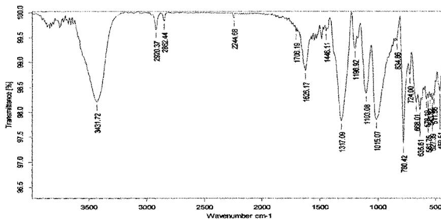
Figure1(a). FTIR spectra of PTh /0.5%w/v V<sub>2</sub>O<sub>5</sub> composite thin films.
